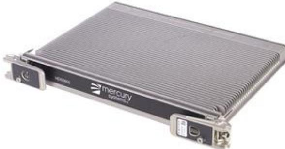
Mercury's new EnsembleSeries™ HDS6605 blade server, the embedded computing industry's most powerful, general-purpose processing 6U OpenVPX™ blade server with hardware-enabled support for artificial intelligence (AI) applications
